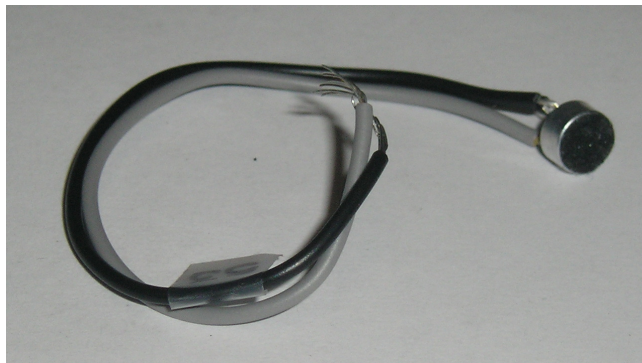
Figure 5-12: A photograph of one 5-mm electret microphone used as an error sensor.
